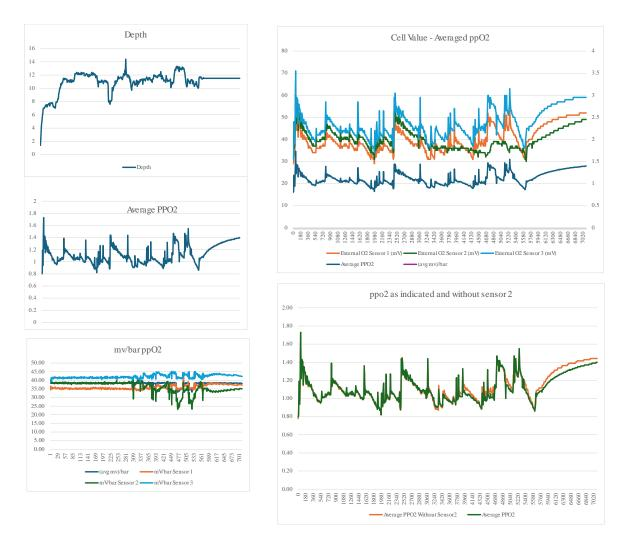
Analysis of previous dives logged indicates some erratic cell behaviour and data indicates Diver 1 potentially conducted some shallow test dives to validate cells. One cell appears to stop working on a dive on 30 January
